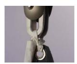
• The tack of the spinnaker shall be attached to the independent swivel with a lashing. If the continuous line furler is not dedicated to one sail, a snap shackle may be used to link the two parts together. The height of the tack is determined by the lashing length.
