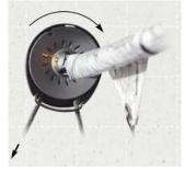
Note: If for any reason a load is too great, the lock is equipped with a fuse that will break and release the continuous line furler.
