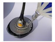
It is also possible to create an adjustable tack line. To do this, you need to attach a block to the independent swivel. We recommend using a soft shackle to attach the tack line. This will make sail changes easier, as well as making it easier to remove the tack line from the unit. When furling, it is important to pull the tack all the way down before furling (tension the luff as much as possible).
