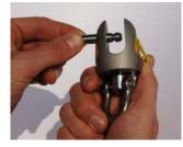
• Install the tack thimble into the drum fork and the head thimble into the top swivel fork.
