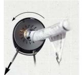
• When the sail is entirely furled, release the continuous line, the drum automatically locks.
