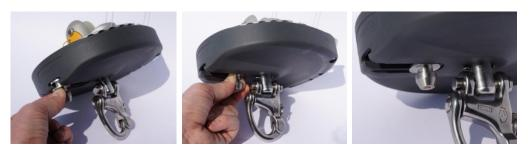
• Check in by furling with your hand if the system works correctly (locks in and locks off when turning the drum in one way, then the other).
