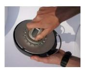
• To remove the lock, pull on the conical piston and slide it out of the drum. The unit will now work in either direction.
