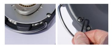
• Remove the cotter pin that holds the spool.
