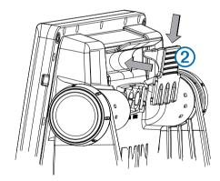
There is an audible click when the locking bracket is installed correctly.
