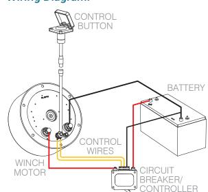
Motor units are supplied with installation manual, control button, 1000mm (39") control button cable, circuit breaker/ controller, cable terminals and terminal extensions.
